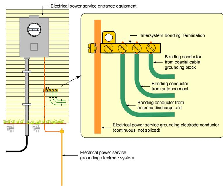
located near the building's electrical service entrance equipment (service entrance equipment typically is a meterbase and main disconnect circuit breaker).
