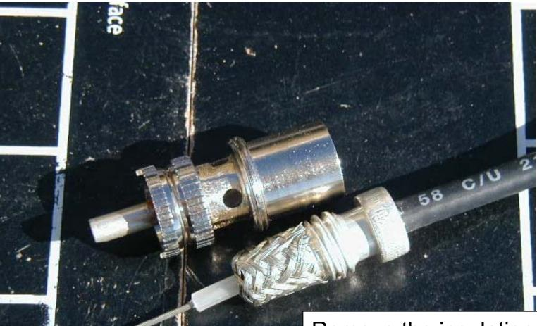
Remove the insulation from the center conductor. Be careful not the nick the center conductor!
